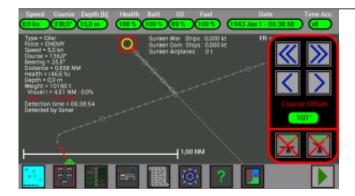
I increase it up to  $101^{\circ}$ , to put my  $2^{\circ}$  circle over the line of the ship, and I will wait for the  $2^{\circ}$  circle of the ship to coincide with my  $2^{\circ}$  circle.
